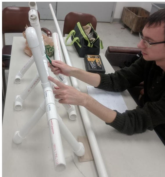
Figure 18: Construction of First Iteration of Agitator
