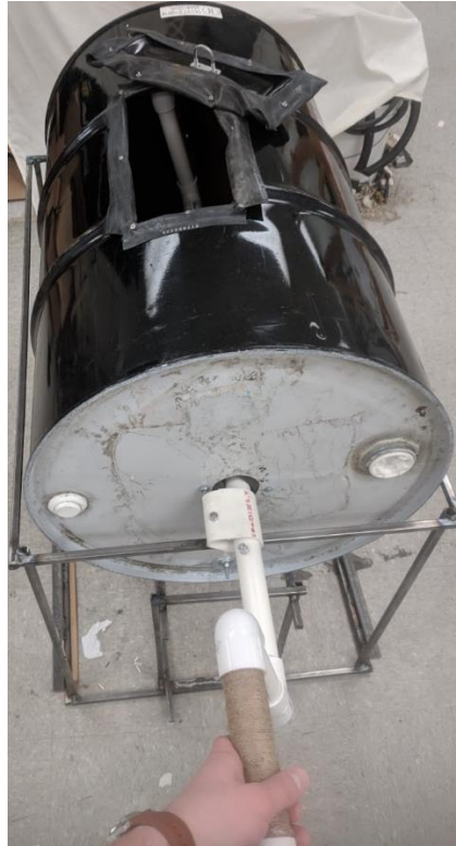
Figure 24: Washing Machine Final Assembly
