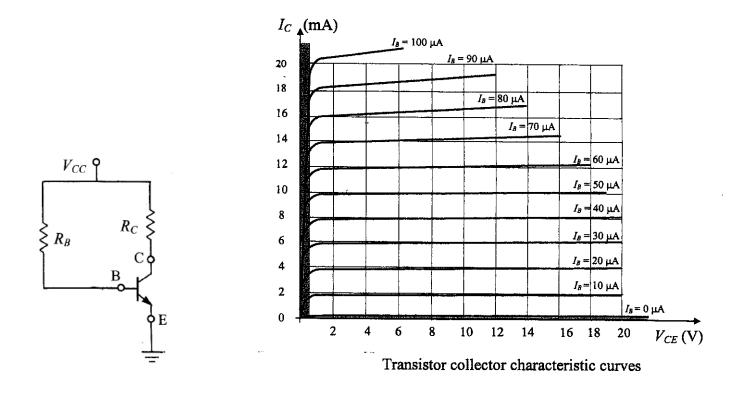
Set the quiescent point at approximately  $I_{CQ} = 8 \text{ mA}$  and  $V_{CEQ} = 9.5 \text{ V}$  with  $V_{CC} = 16 \text{ Volts}$ .
