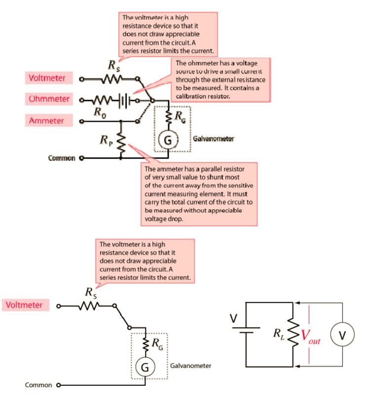
A voltmeter is connected in parallel with the circuit element  $(R_L)$  to measure voltage.
