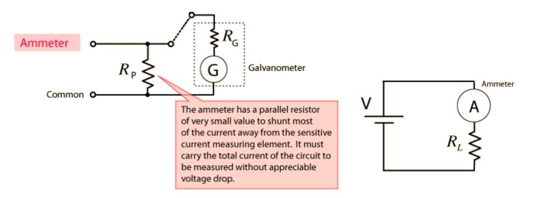
A ammeter is always connected in series with the circuit element  $(R_L)$  to measure current.
