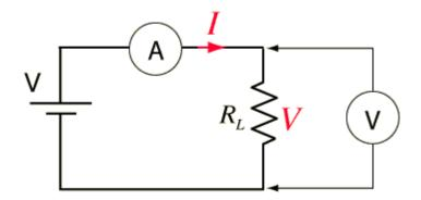
The Resistance  $R_L$  equal to  $R_L = \frac{V}{I}$
