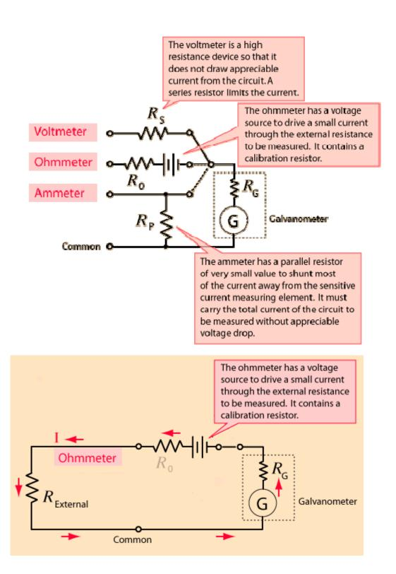
The circuit element  $(R_L)$  must be disconnect from the circuit in order to measure resistance with an ohmmeter.
