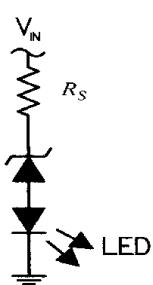
Calculate Minimum Input Voltage
