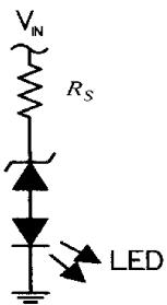
$$\begin{aligned} R_s &= 220 \Omega \\ V_{Zener} &= 2.7 \text{ V} \\ I_{LED} &= 15 \text{ mA} \end{aligned}$$
