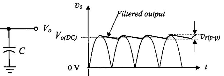
$$V_{\text{ripple(peak- peak)}} = I_{\text{out(DC)}} / 2fC$$
