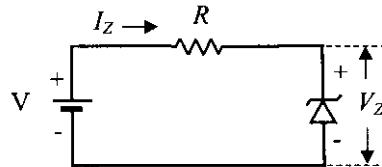
If  $V_{\text{Source}} > V_Z$  then  $V_0$  maintained at  $V_Z$ , else  $V_0 = 0$
