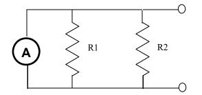
$$I_{R_2} = I \ \frac{R_1}{R_1 + R_2}$$
