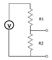
$$V_{R_2} = V \frac{R_2}{R_1 + R_2}$$
