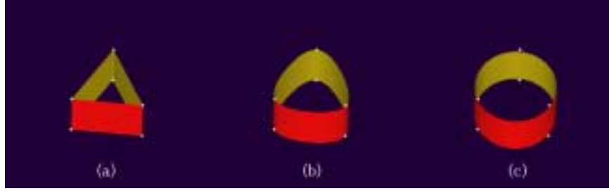
Figure 3: The half-closed RaG surface interpolating the vertices of two parallel equilateral triangles falls between the polyhedron obtained by connecting the triangle vertices and the cylinder that interpolates the polyhedron. (a) \sigma = 0.01 . (b) \sigma = 0.2 . (c) \sigma = 0.5 .
